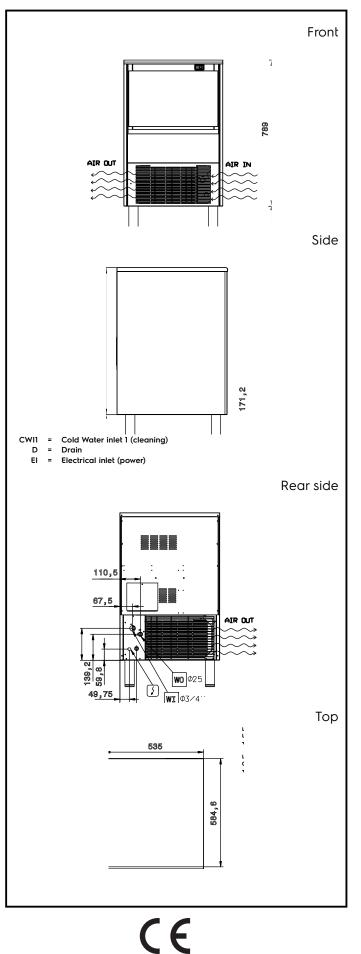
Ice Makers Ice Cuber (22gr), 55kg/24h, 25kg bin, air-cooled - drain pump
